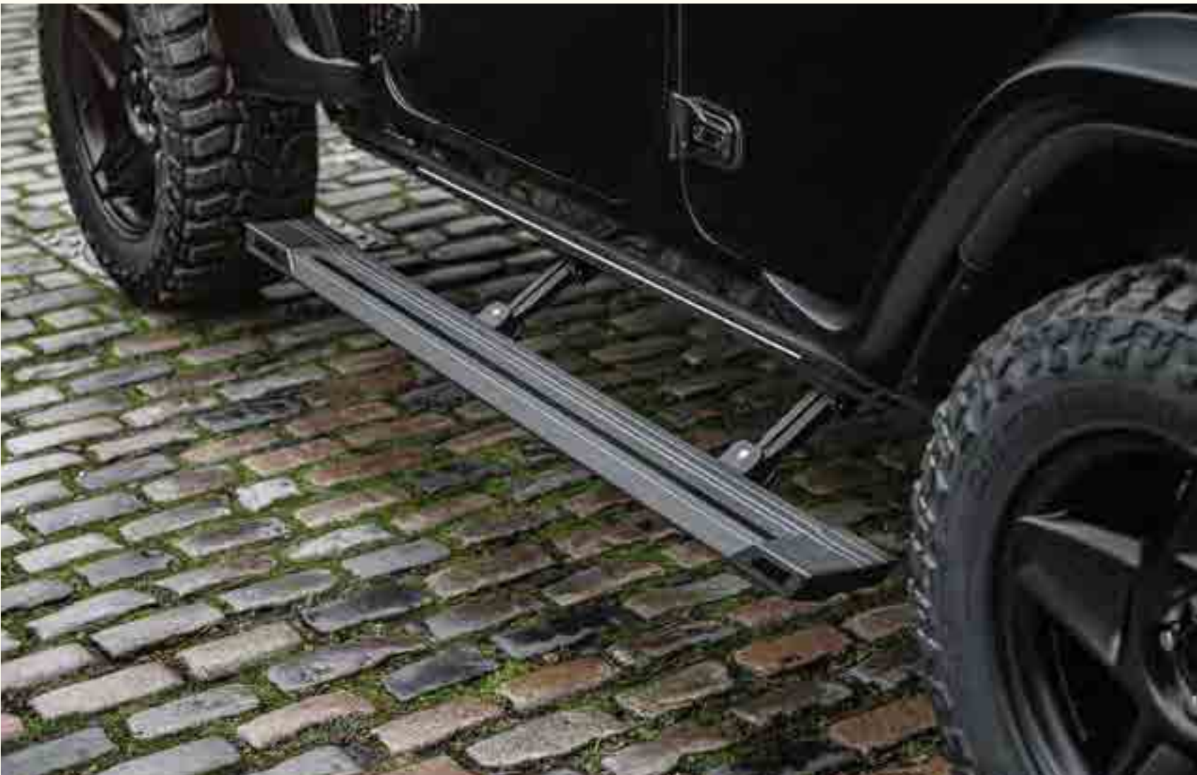
4 DOOR ELECTRIC SIDE STEPS WITH LIGHTS (RUNNING BOARDS) PART NUMBER: KSJMNBN
