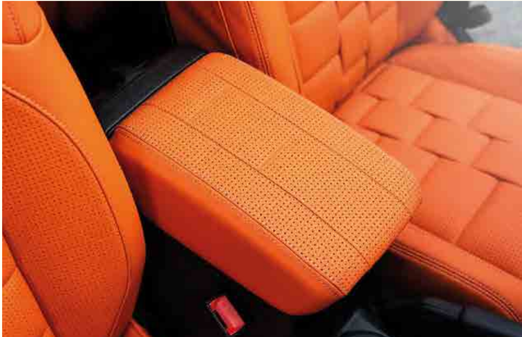
CENTRE GLOVEBOX COLOUR: VOLCANIC BURNT ORANGE CENTRE GLOVEBOX: REUPHOLSTERED IN LEATHER PART NUMBER: L129679
